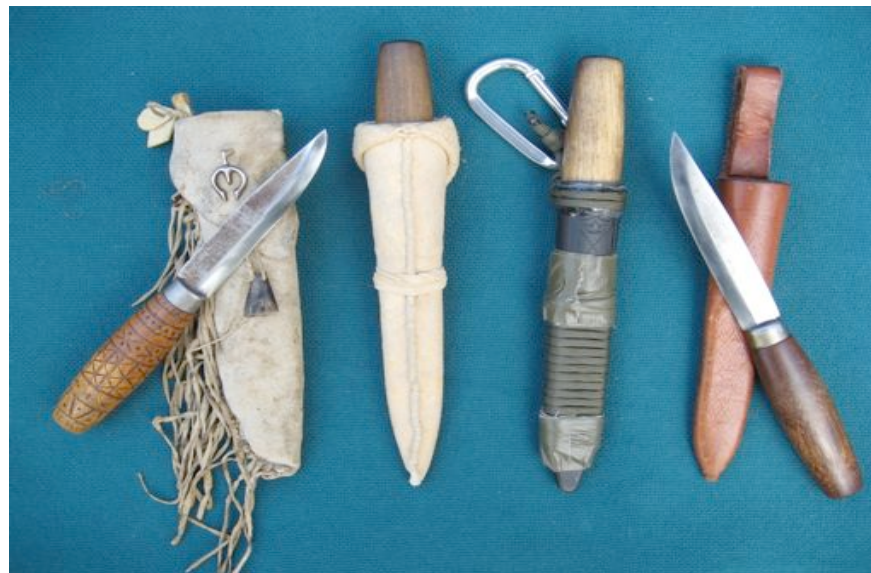
A classic tool: The 4-inch laminated carbon steel Mora knife, shown with sheath options. From left to right: An early effort at buckskin covered rawhide sheath construction, with awl and attached decorations visible at top of sheath; buckskin covered plastic sheath, using rawhide extension discussed in text; plastic sheath with extra cordage wrapping and snap ring; original Mora leather sheath.
