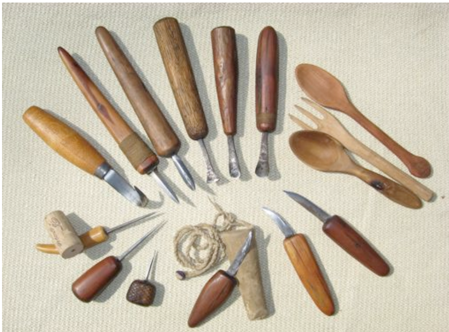
Awls, crooked and curved knives, gouges, and small knives are useful for a wide range of tasks. Crooked knife (left center) by Mora. Blade of curved knife (above Mora crooked knife) made by Kestrel tool. All other tools by the author. Cork (lower left) is placed over tip of awl when not in use, protecting both tool and user.
